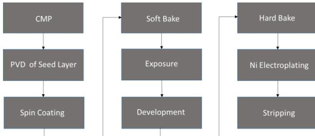
Fig. 7 Process steps of mold inlay
