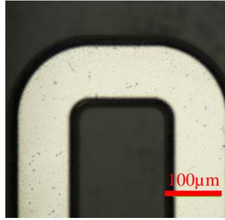
Fig. 15 Polished sputtered micro structure I
