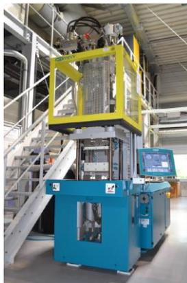
Fig. 11 Injection molding machine Dr. BOY 55EVV<sup>®</sup>
