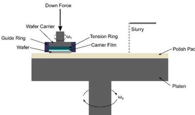
Fig. 10 Schematic CMP process
