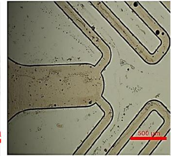
Fig. 13 Electroplated Ni structure on injection mold inlay
