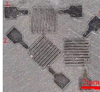
Fig. 19 Manufactured Pt-sensors
