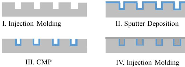
Fig. 1. Process steps for sensor array (cross section)
