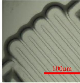
Fig. 17 Injection molded PC structure
