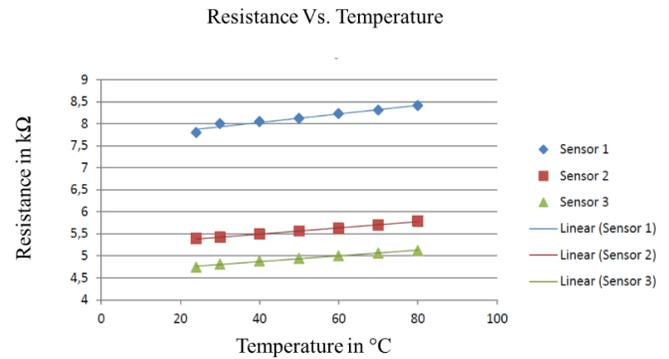
Fig. 21 Resistance vs. Temperature behavior of the Pt-sensors
