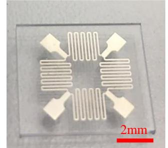
Fig. 20 Wheatstone bridge on PC-substrate
