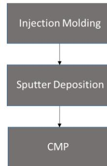
Fig. 14 Sensor manufacturing process steps (demonstrator)
