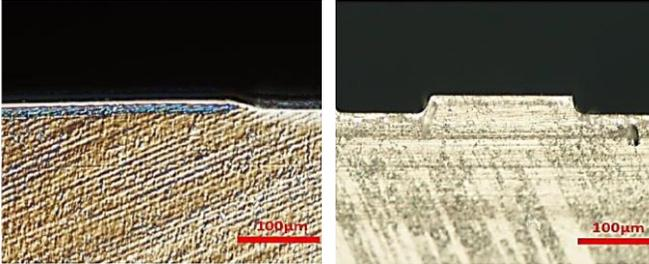
Fig. 8 Cross section of 100 nm structure height (reflected-light microscope)
