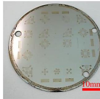
Fig. 12 Manufactured injection molding inlay
