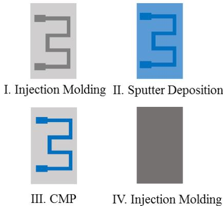
Fig. 2. Process steps for sensor array (top view)
